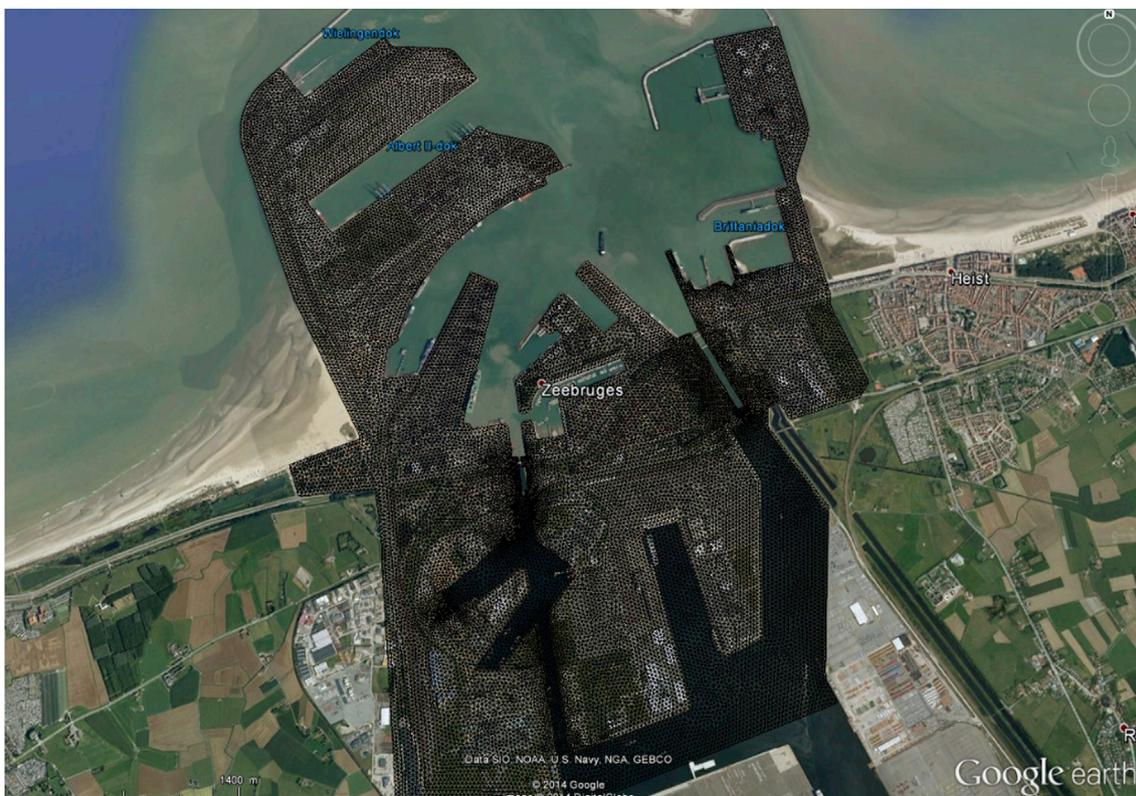
Fig. 4. TELEMAC model for the harbour of Zeebrugge case study site (the small black dots are the grid points of the model).
